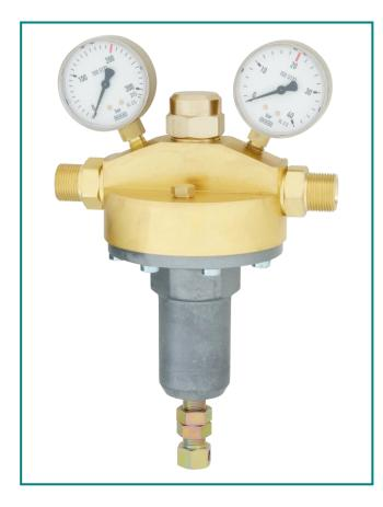
Central pressure regulators or main pressure regulators, describes pressure reduction valves that reduce the high pressure from main containers (compressor tanks, cylinder batteries or liquid gas tanks) to an intermediate pressure. The amount of intermediate pressure depends on the gas volume and pressure that would be needed by the following gas supply station.
